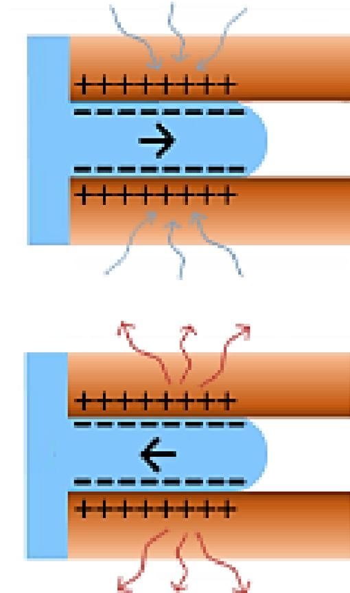
**Porous materials with 500 – 2000 m<sup>2</sup>/g are typically used for intrusion-extrusion.
