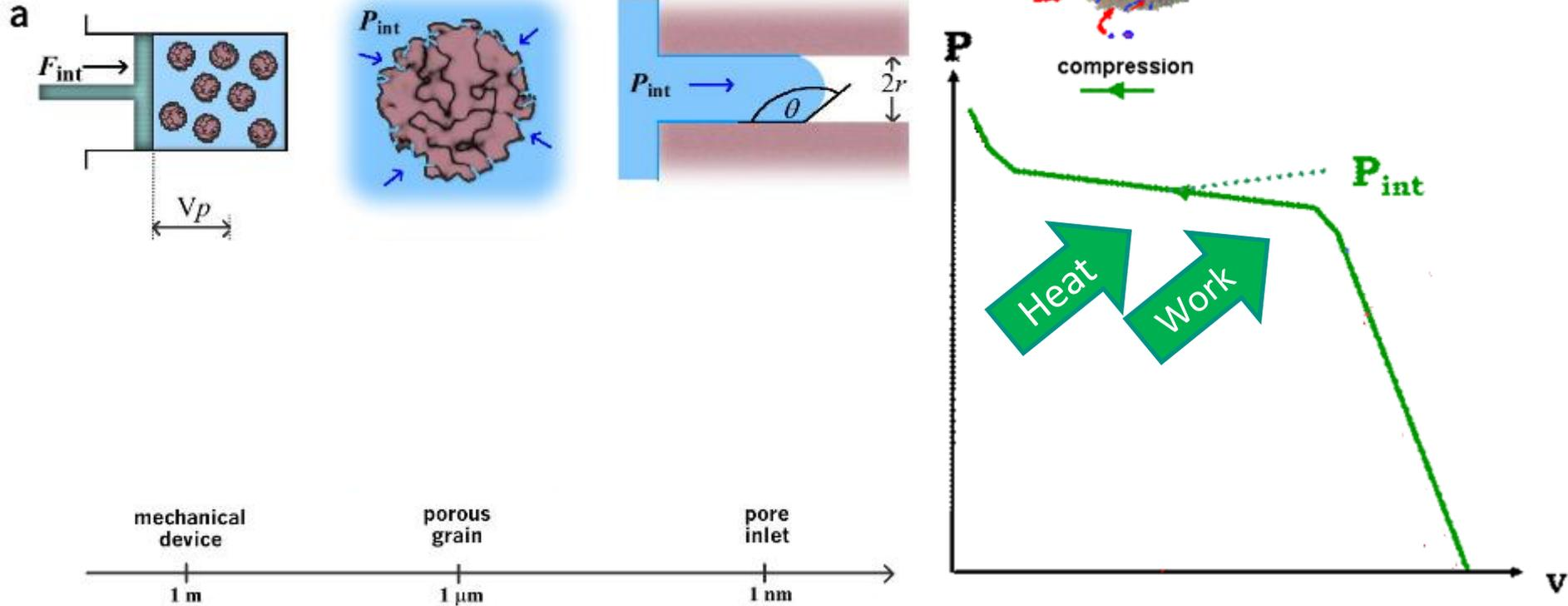
$$W_{intrusion} = P_{intrusion} \cdot \Delta V = P_{intrusion} \cdot V_{pores}$$
