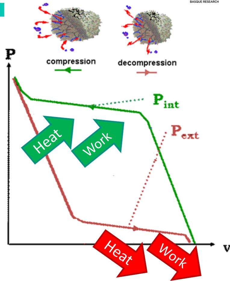
$$W_{intrusion} = P_{intrusion} \cdot \Delta V = P_{intrusion} \cdot V_{pores}$$
